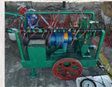
Load the Super Cell by hydraulic pump
